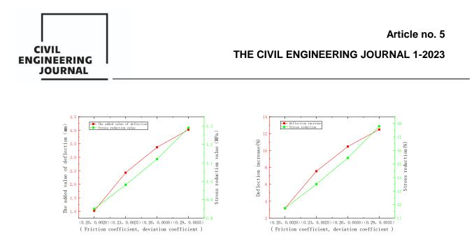
Fig. 16 - Coupling changes of friction coefficient and deviation coefficient on deflection and stress of main beam Influence diagram
