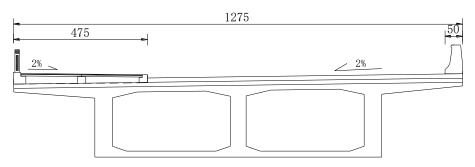
Fig.2 - Bridge cross section (Unit: cm)
