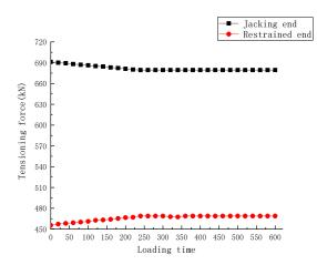
Fig.11 - Relationship curve between load holding time and tension of F1b steel
