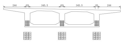
Fig.3 - Layout drawing of prestressed steel beams (Unit: cm)
