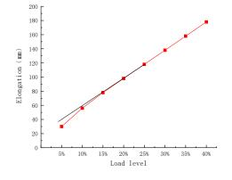
Fig. 10 - F3e tension and elongation relationship curve
