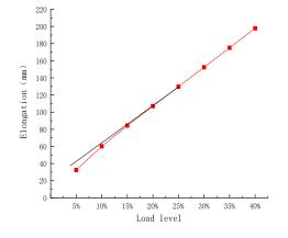
Fig. 9 - F1b Tension and elongation relationship curve
