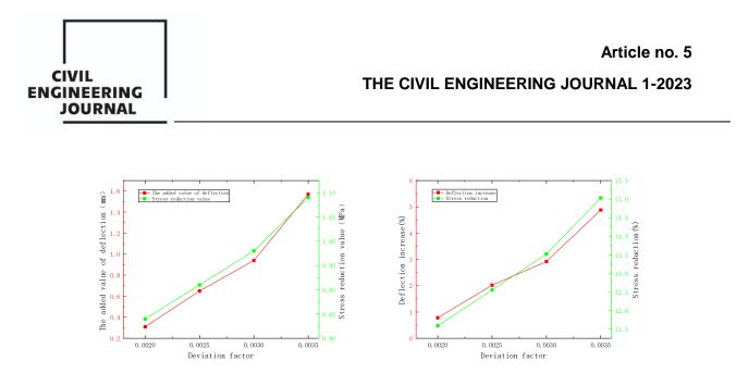
Fig. 15 - Influence diagram of deviation coefficient alone changes on deflection and stress of main beam
