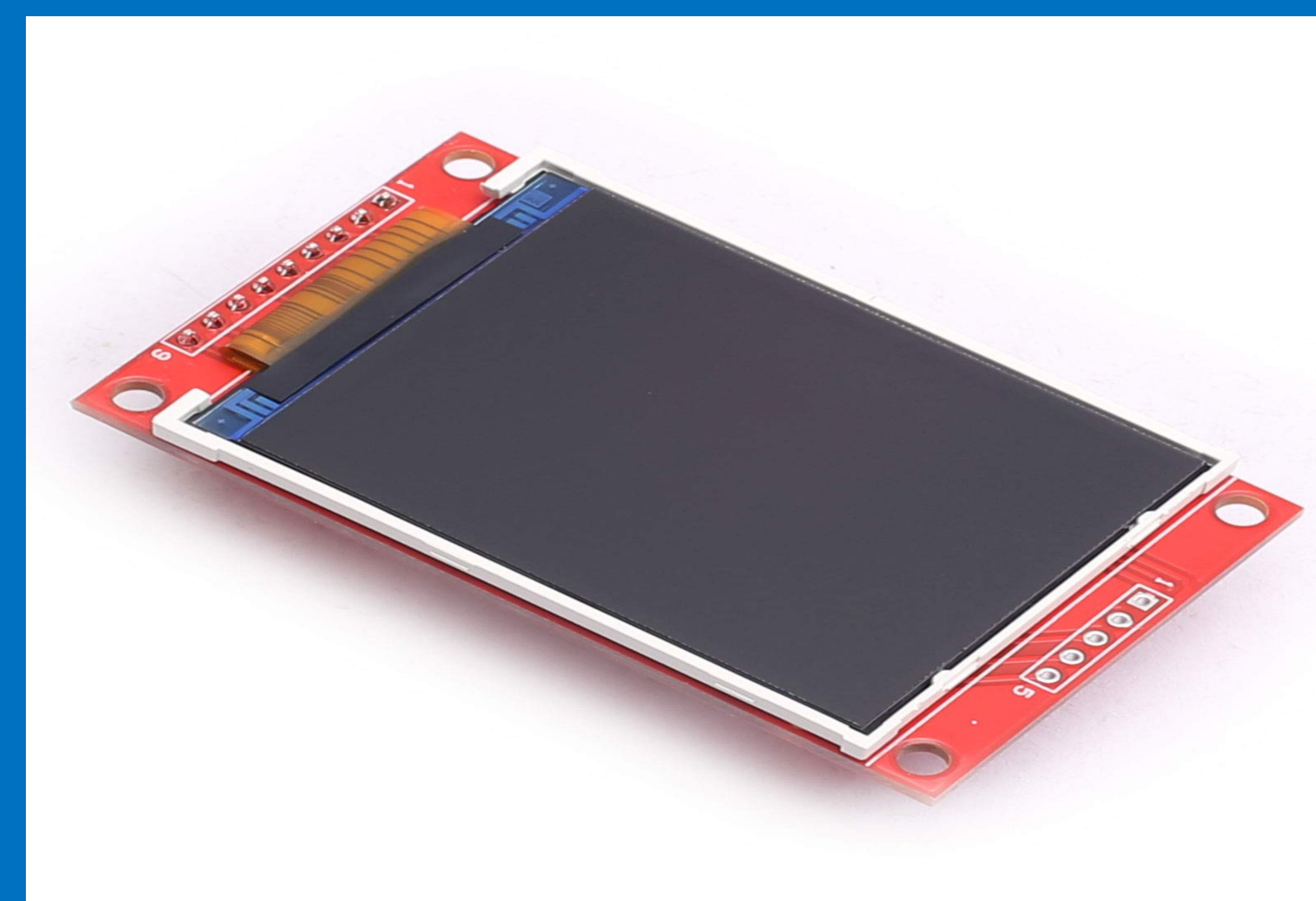
Figure 3. ILI9341 2.2" LCD screen with SD card
