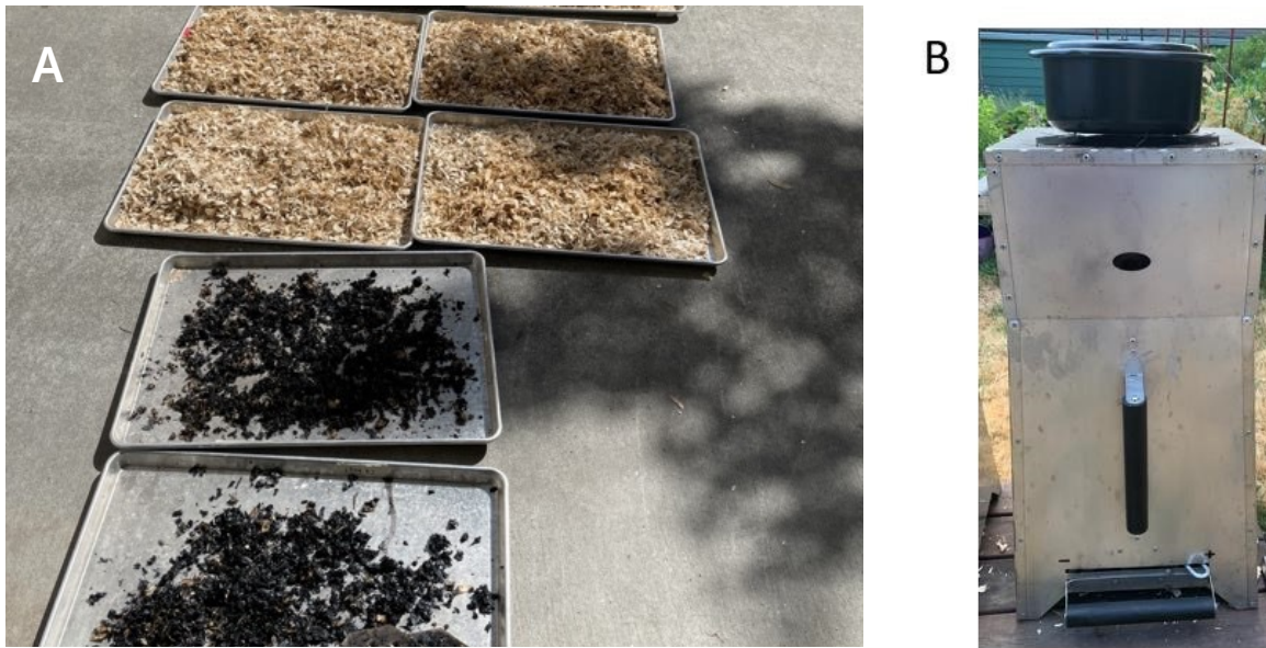
Figure 1 (A) Aspen wood chips drying outdoors and pyrolyzed biochar. (B) Low-emissions biochar cookstove.
