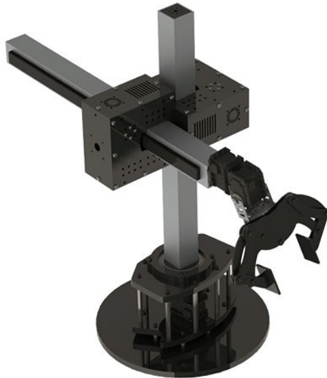
Figure 28: Cylindrical robotic arm (Articulated Robotic Arm, 2020)
