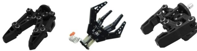
Figure 36: Example of servo grippers (NIRYO NED ROBOT, 2022)
