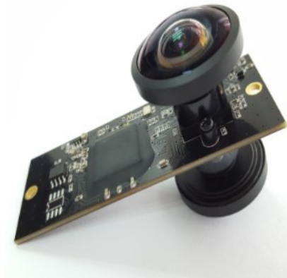
Figure 56: 360° VR Panorama Dual lens Camera Module with Micron MI0130 sensor
