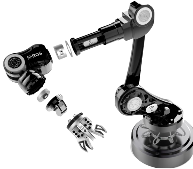
Figure 11: Modular robot design example (Uraga, 2017)
