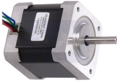
Figure 62: Typical stepper motor 200 Steps/Rev, 42×48mm, 4V, 1.2 A/Phase 0.35kg. Cost around 20 €
