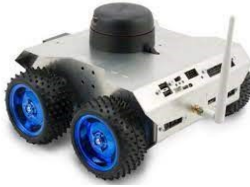
Figure 4: Wheeled robot (SOFFAR, Wheeled robots types, uses, advantages and disadvantages, 2019)
