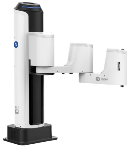
Figure 26: SCARA Robotic Arm example (DOBOT M1, 2022)
