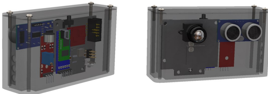
Figure 86: Side electronics in their box. Three of them, identical, will be place on the robot.
