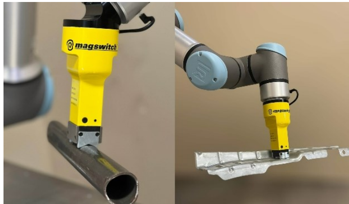
Figure 38: Magnetic gripper examples (Robot Enthusiast, 2022)
