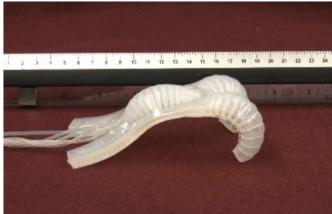
Figure 10: Soft elastic robot (Jablonski, 2011)
