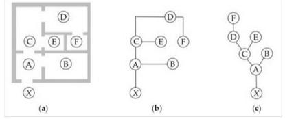
*Fig. 5.* Example of justified graph map: (a) Architectural layout with six rooms, annotated A–F, with the exterior (X) as carrier; (b) diagram shows the connections between the spaces; (c) justified graph of the plan. (Ostwald & Dawes, 2018, p. 55-56)
