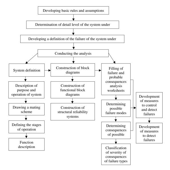
Figure 1. Scheme of the analysis of failures and their consequences.
