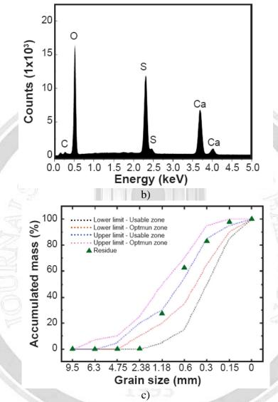
Figure 1: (a) SEM Micrograph, (b) EDS Spectrum of the Gypsum Waste Powder, and (c) Curve of Particle Size Distribution [3].
