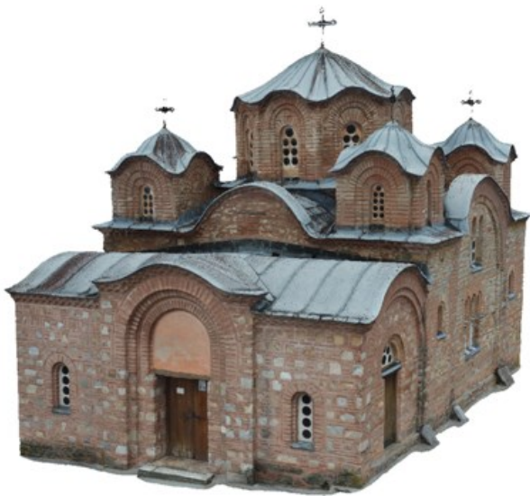
Figure 6. Final photogrammetric model combined with laser scanned data for getting of correct scale of the model (Agisoft Metashape and RealityCapture).
