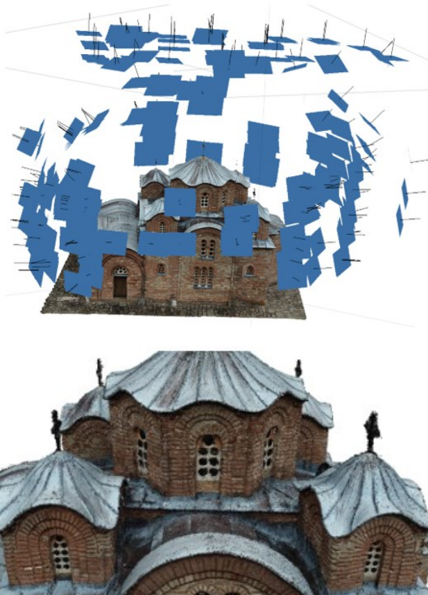
Figure 3. Drone photogrammetry and the upper part of the church model.
