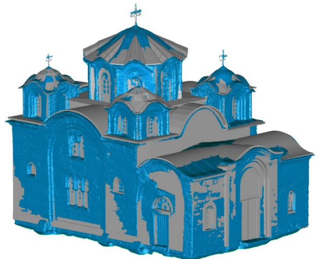
Figure 15. Comparison of both 3D models: BIM geometrical basic model (grey), photogrammetrical model (blue).
