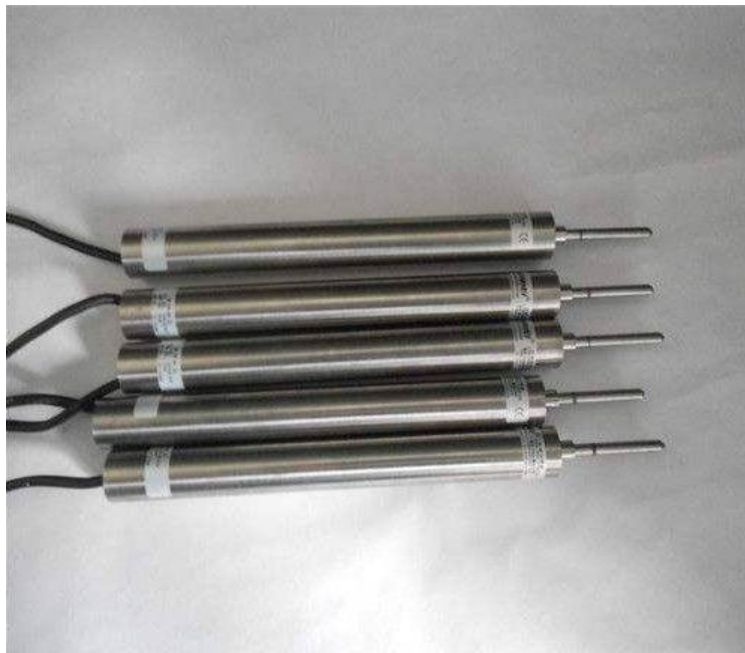
Fig.6. D020 displacement sensor
