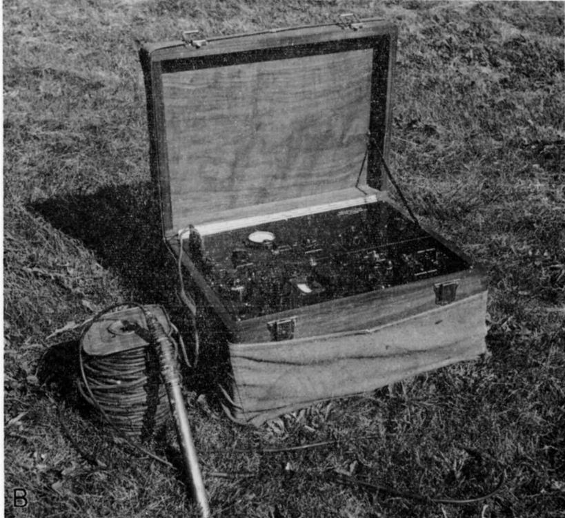
PLATE 2. A , Set-up of resistivity equipment in field operation. B , Electrical resistivity instrument and the logging device. (Photo by Ada Swineford)
