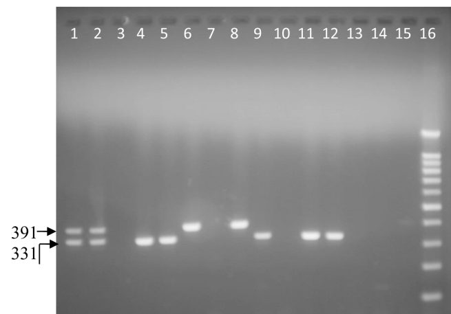
Figure 1. Ethidium bromide stained 1.5% agarose gel electrophoresis of Campylobacter coli (391 bp) and C. jejuni (331 bp) in a multiplex PCR with a 100-bp ladder. From left to right, lane 1 and 2 positive samples; mixture of Campylobacter jejuni and Campylobacter coli obtained from sequenced laboratory isolates (PHPT 1 & 2). Lane 3 negative control: purified water. Lanes 4, 5, 9, 11 and 12: C. jejuni . Lanes 6, 8 and 15: Campylobacter coli . Lanes 7, 10, 13 and 14: negative samples. Lane 16: 100-bp ladder.
