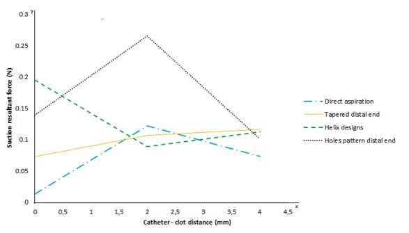
Figure 7. Plot for suction pressure vs clot distance for the series of designs.
