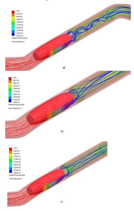
Figure 4. Pressure distribution for a given experiment: (a) Helix, (b) Holes pattern and (c) Cone.
