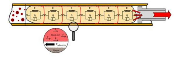
Figure 3. Damped mass-spring system with 6 DOF.
