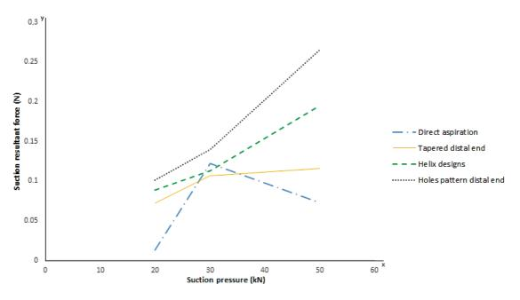
Figure 6. Plot for suction pressure vs force for the series of designs.
