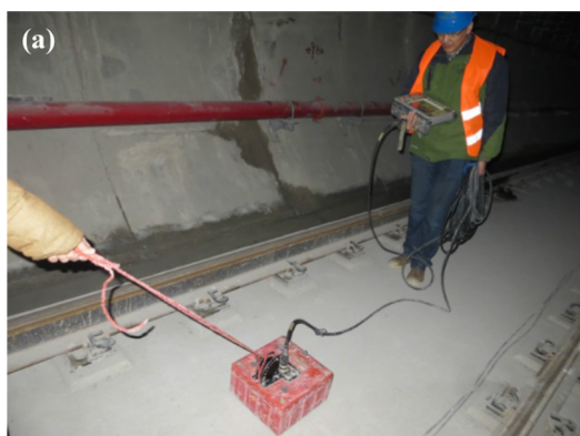
Fig. 8. Photos showing the GPR scanning of the tunnel: (a) Scanning of tunnel floor, (b) Scanning of tunnel roof.
