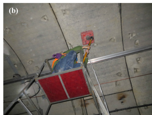
Fig. 8. Photos showing the GPR scanning of the tunnel: (a) Scanning of tunnel floor, (b) Scanning of tunnel roof.
