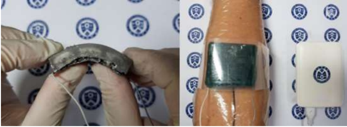
Fig. 97: The flexible hydrogel-based heatsink fabricated onto the TEG [274].
