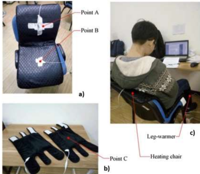
Fig. 18: The personal heating devices: a) the heating chair; b) the leg warmer; and c) a subject using the devices [104].
