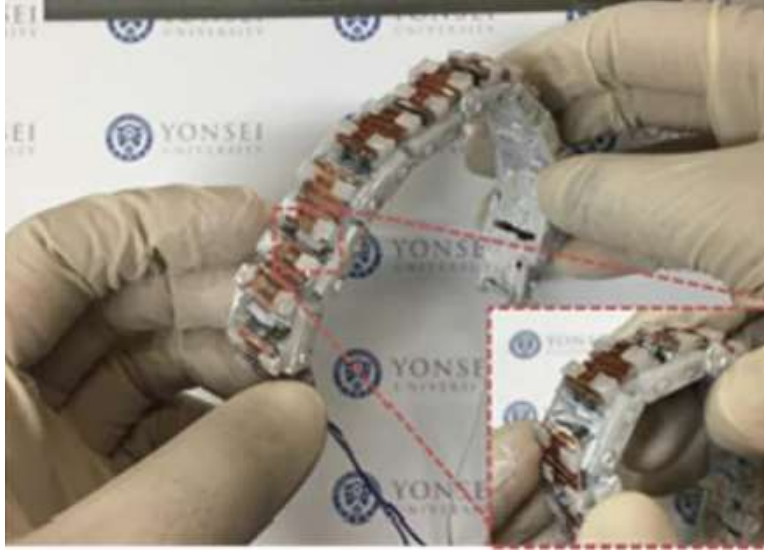
Fig. 44: The designed flexible TE system consisted of a flexible holder [248].
