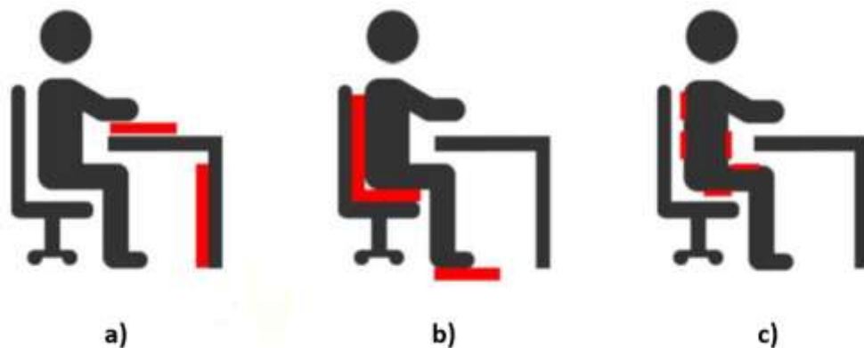
Fig. 17: The heating strategies used in this study: a) HB1: a radiant heating panel with a heated table pad; b) HB2: a heated chair with a heated floor mattress; and c) EHC: a heated jacket with heated trousers [22].
