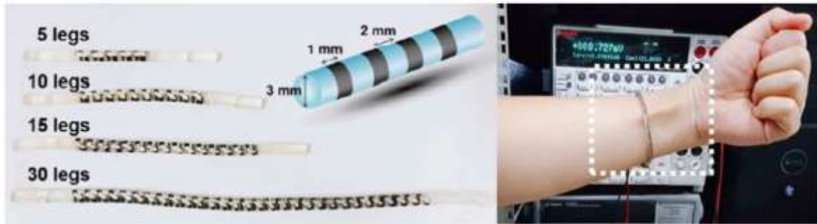
Fig. 51: Photograph of the devices with 5, 10, 15 and 30 PN pairs. Demonstration of the TE bracelet wrapped around the wrist [285].
