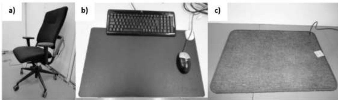
Fig. 16: The fabricated personalized heating systems: a) a heated chair; b) a heated desk mat; and c) a heated floor mat [10].
