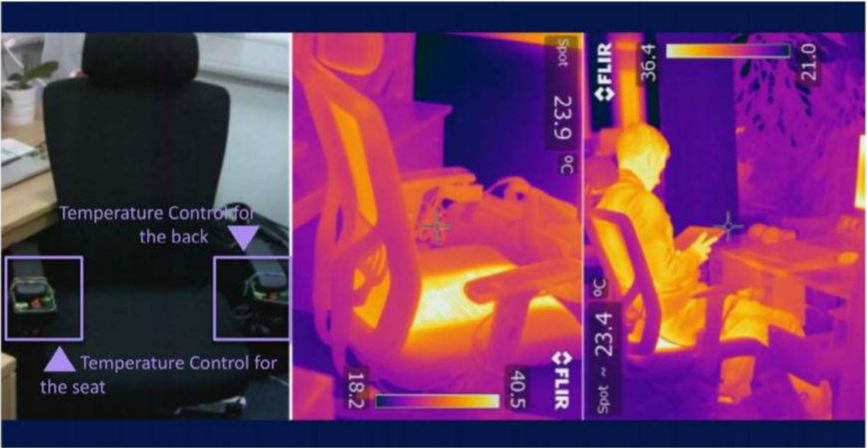
Fig. 12: The design and the thermal image of the heating chair [95].
