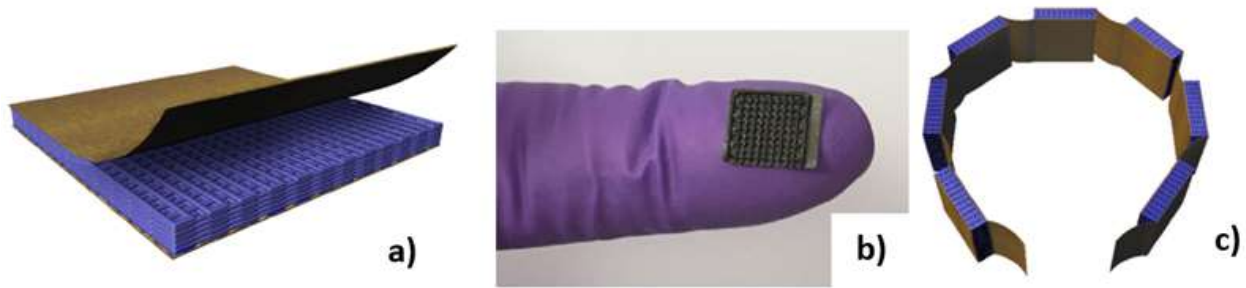
Fig. 52: a) The schematic of the 3D printed PDMS grid; b) Photo of the fabricated grid-based TEG; and c) Schematic design of integrating 7 units of the developed grid-based TEGs together [286].
