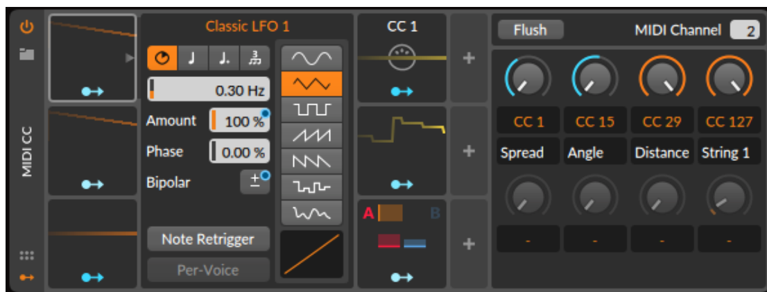
Figure 16 Bitwig's Classic LFO configured for a single string in GASP system, to provide control for the multiple parameters of Spread, Angle and Distance spatialization.
