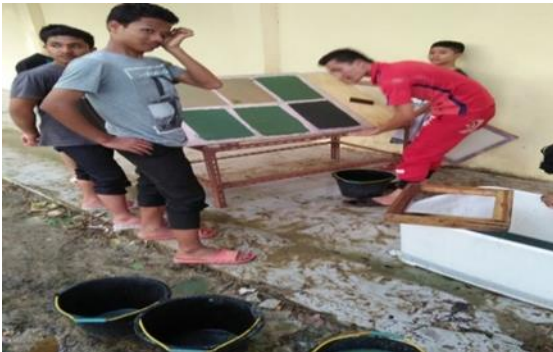
Fig. 11. Adjusting the pulp screen to triplex on a sloping table
