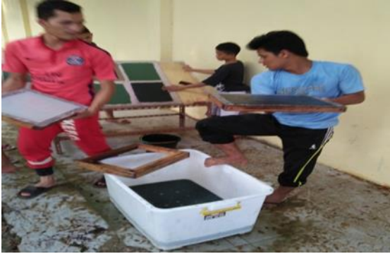
Fig.10. Lifting the screen of pulp paper
