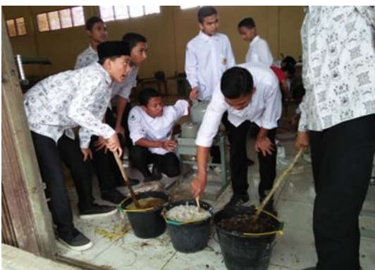
Fig. 6. Stirring the soaked pulp raw materials
