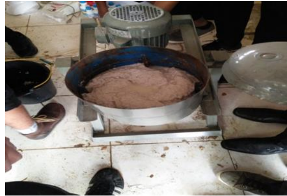
Fig. 7. Pouring pulp into big blender
