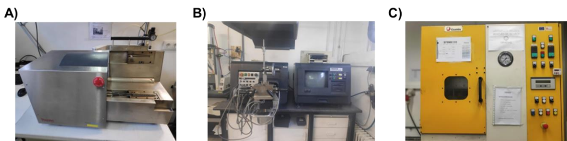
Figure 4.5. Equipment used for materials processing. A) Mini-extruder, B) Internal mixer, C) Automatic platen-press
