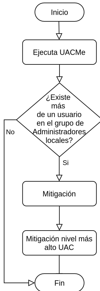
Figura 4.6: Control de flujo de la técnica Bypass User Account Control
