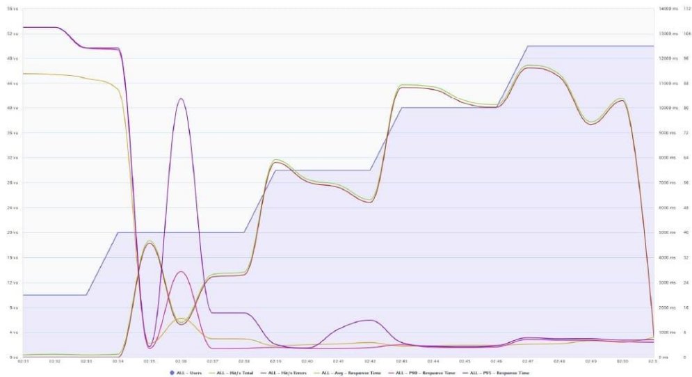
FIGURE 4. Microservice performance patterns for SPIDEPMS-T2-SQL (second scenario). The coloured lines represent various parameters: blue: active connections (vu); light green: request/hits per second; red: error/hits per second; light orange: average response time; magenta: 90th percentile response time; purple: 95th percentile response time.
