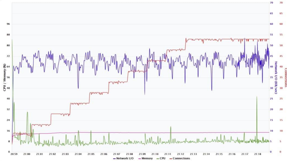
Figure 4. Engine Health Report SPIDEP-SOA-K8s-T1. The colored lines represent various parameters as follows: the blue line is the bandwidth traffic; the purple line is the memory load generated by the users; the green line is the CPU load generated by the users; and the red line is the active connections within the test.
