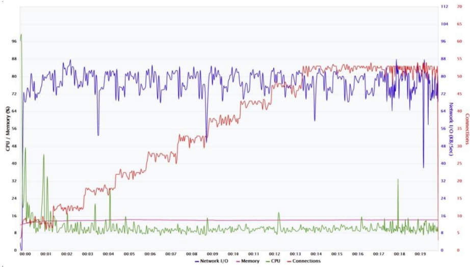
Figure 7. Engine Health Report SPIDEP-MSA-K8s-T2. The colored lines represent various parameters as follows: the blue line is the bandwidth traffic; the purple line is the memory load generated by the users; the green line is the CPU load generated by the users; and the red line is the active connections within the test.
