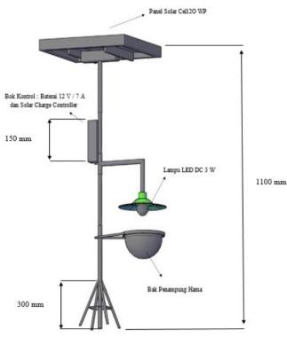
Figure 1. Pest Trap Design
