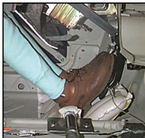
Abb. 5-23 Lower leg Airbag [21]
