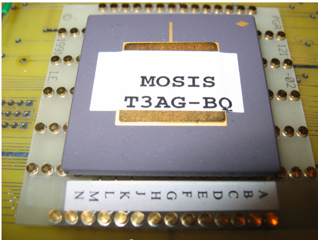
Figure 109: One out of 15 chip exemplars which were received from the MOSIS chip manufacturing service. It is located on an Ironwood-121 prototyping adaptor.
