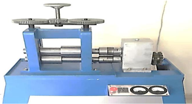
Figure 2. Asymmetric flat rolling machine with two various roll diameter ratios.
