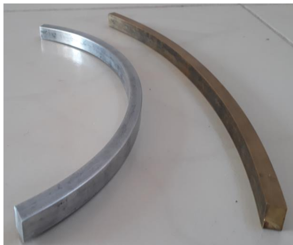
Figure 5. The aluminum and brass bars after the asymmetric rolling process
