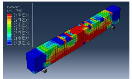
Figure 24. The pattern of cracks in the beam made of RC having rebars of 25 mm diameter
