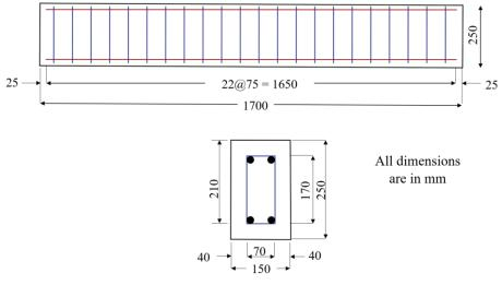
Figure 1. Details of the reference reinforced concrete beam
