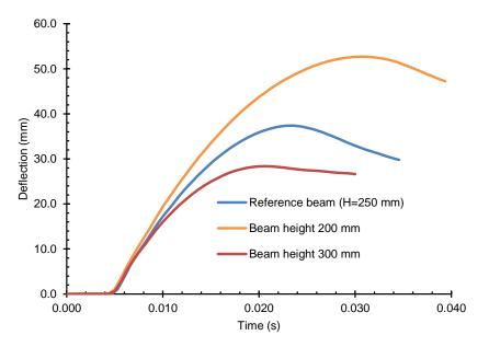
Figure 16. Effect of the beam depth on deflection-time history
