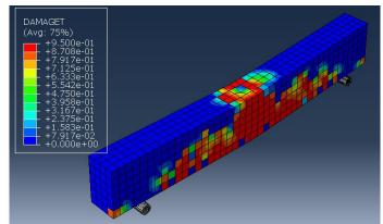
Figure 5. Crack pattern of the reference beam at impacting loading
