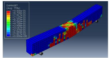
Figure 22. The pattern of cracks in the beam made of RC having rebars of 12 mm diameter
