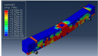
Figure 17. The pattern of cracks in the RC beam with 200 mm depth
