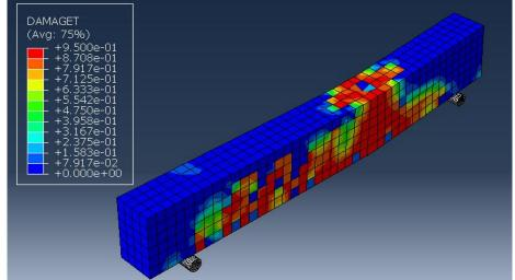
Figure 14. The pattern of cracks in the RC beam subjected to eccentric impacting loading
