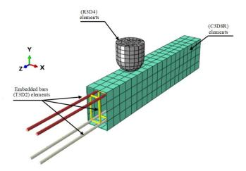
Fig. 2. Details of the finite element mesh utilized for concrete beam modeling
