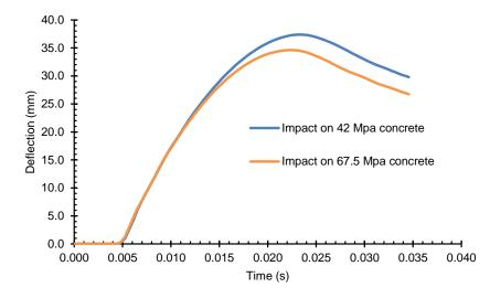
Figure 10. The deflection-time history as affected by the of the concrete strength in comp.
