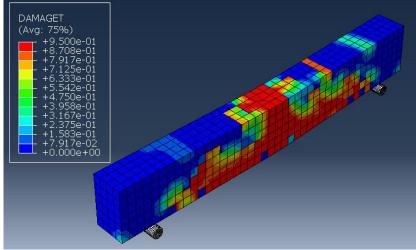
Figure 23. The pattern of cracks in the beam made of RC having rebars of 20 mm diameter
