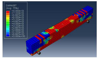
Figure 8. The pattern of cracks in the RC beam with FRP reinforcement bars
