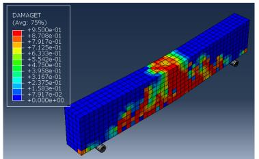
Figure 18. The pattern of cracks in the RC beam with 300 mm depth
