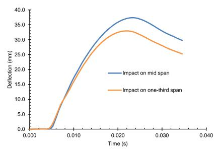
Figure 13. Effect of the location of impacting weight on the deflection-time history
