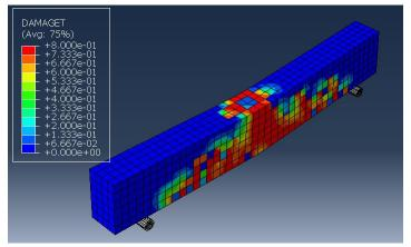
Figure 11. The pattern of cracks in the RC beam with high strength concrete
