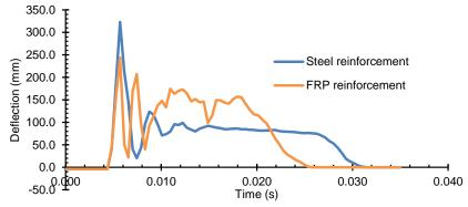
Figure 6. Effect of FRP reinforcing bars on impact force-time history
