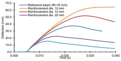
Figure 20. Effect of different reinforcing diameter on deflection-time history
