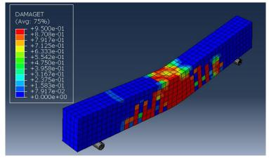
Figure 21. The pattern of cracks in the beam made of RC having rebars of 10 mm diameter
