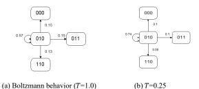
Fig. 7. Transition probabilities for different temperatures.
