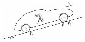
Fig. 1. Resistance forces acting on a moving car on a slope.
