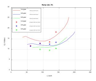
Fig. 9. Fuel consumption in third, fourth and fifth gear at 4% slope.
