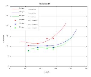
Fig. 8. Fuel consumption in third, fourth and fifth gear at 2% slope.
