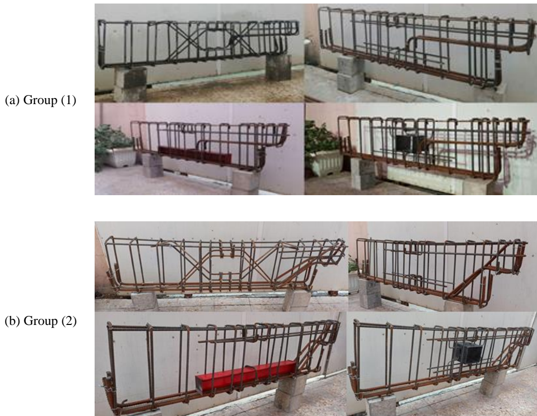
Fig. 8 – Reinforcement of Dapped and Beams with openings
