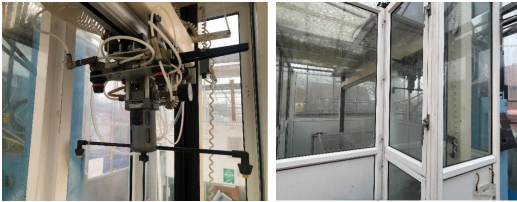
Figure 2.2.1 The customized built-in pot sprayer inside an enclosed chamber with a pair of nozzles.
