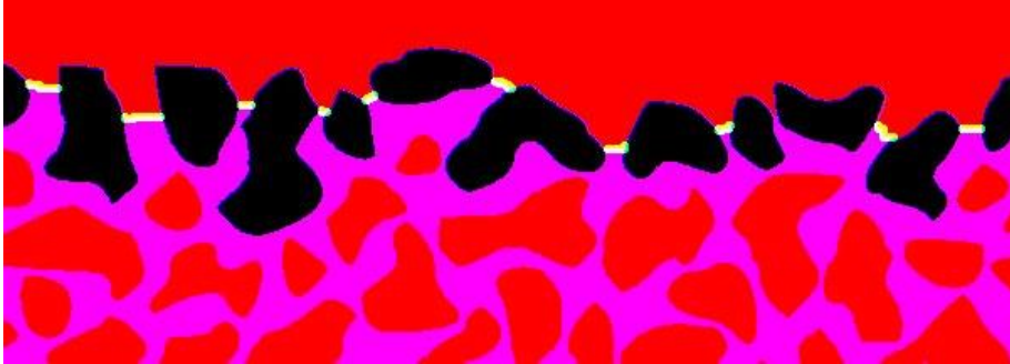
Figure 5. 1 The equivalent square capillary width d_0 of MM4 is determined by the pore throats of the first layer grains (marked in yellow).
