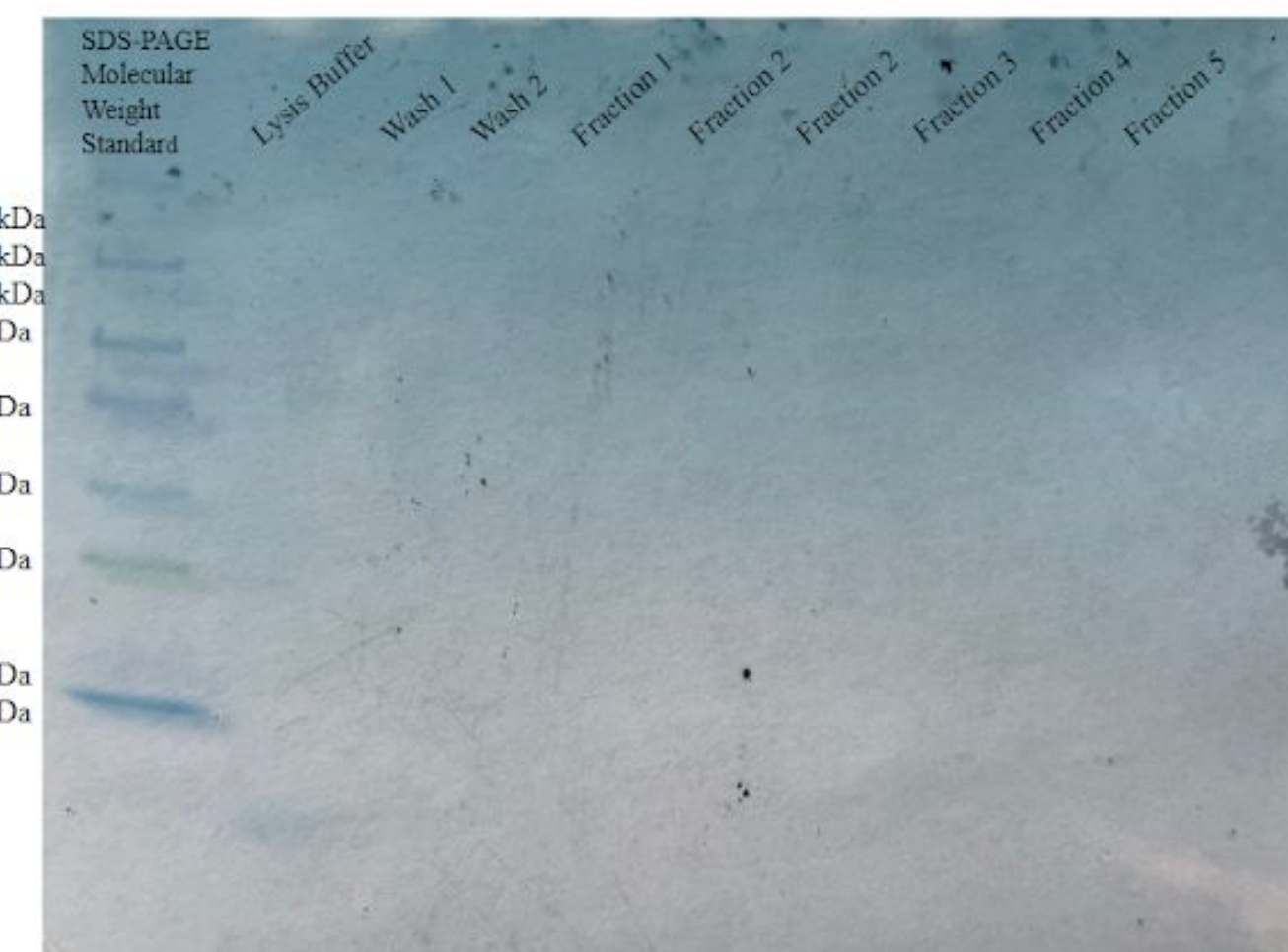
Figure 5. Coomassie Stained Sodium Dodecyl Sulfate PolyAcrylamide Gel Electrophoresis. Samples were analyzed by adding 30 µl of each sample to 10 µl of 4x SDS buffer sample in order to denature. This was followed by heating the samples for 5 minutes on a 100°C heat block and then onto a 4-20% polyacrylamide gel alongside a molecular weight marker. The gel was run for 1 hour at 150V and then stained in coomassie stain.
