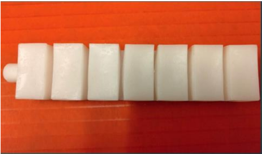
Fig. 9: SLA printed soft robotic gripper.
