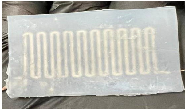
Fig 22: The physical diagram of the preparation process of the liquid metal sensor.
