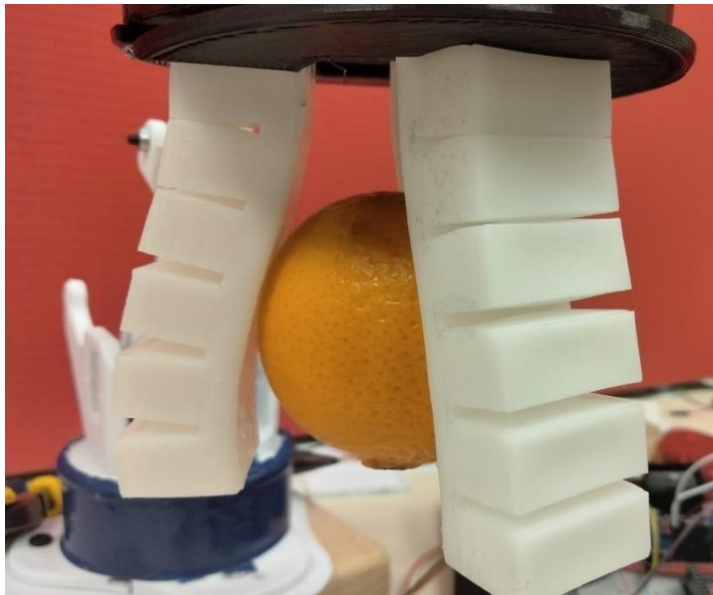
Fig 13: Optimal grasping position of Orange at the applied pressure of 80 KPa
