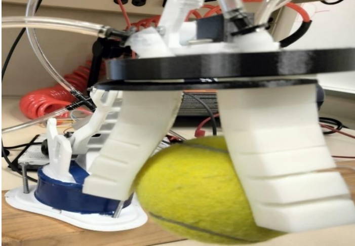
Fig 14: Optimal grasping position of the Ball at the applied pressure of 100 KPa.
