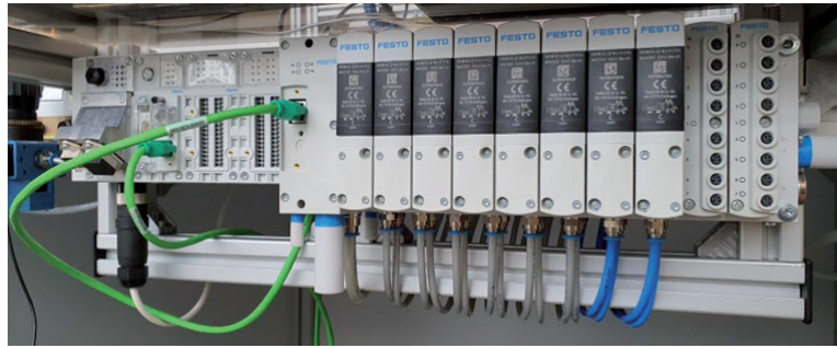
Fig. 6. FESTO Motion Terminal, with an 8-valve configuration for up to 16 parallel pneumatic outputs.
