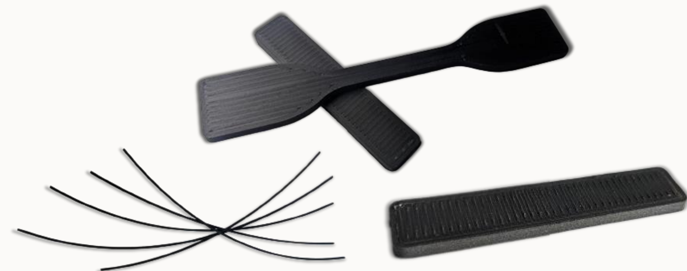
Figure 1: CPC filament and mechanical test samples.
