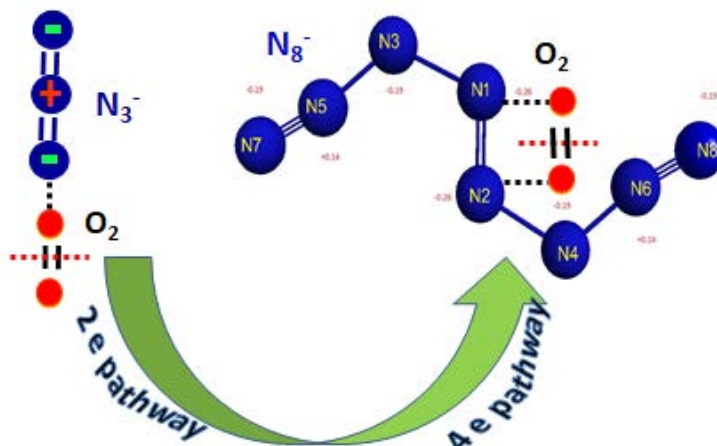
Figure 2.8 Mechanism for oxygen reduction on N_3^- and N_8^- based on different O_2 chemisorption mode.
