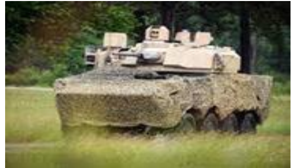
Gambar John Cockerill 3030 Unmanned Turret Sumber: Johncockerillda.com
