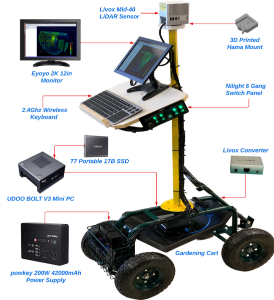
Fig. 1: Prototype of portable AQ LiDAR device.
