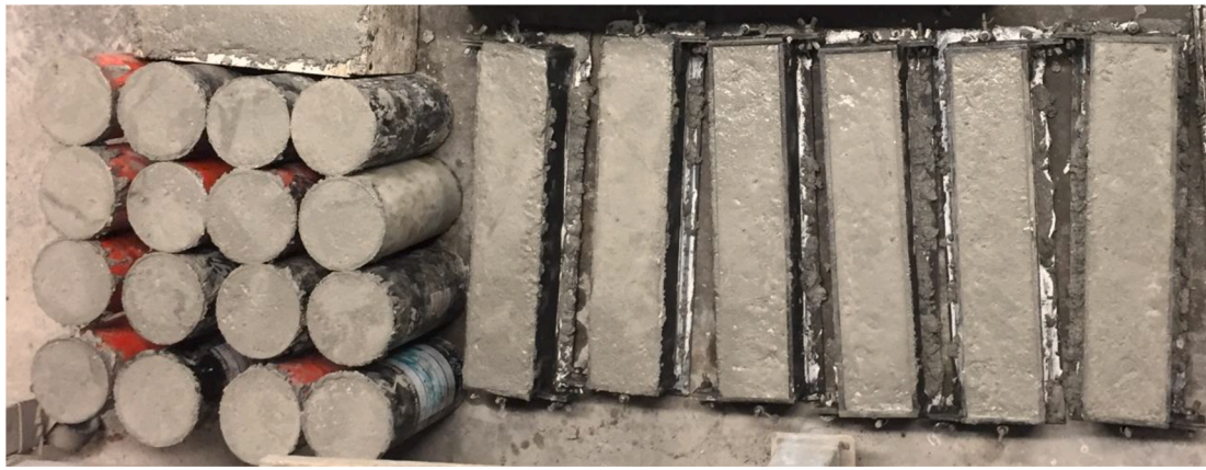
Fig. 2. WLP concrete specimens after casting.
