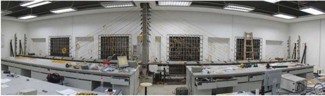
Fig. 3. The 1/40 scale model of a cable-stayed bridge.
