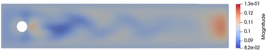
Fig. 12 Algorithm (4) solution when \epsilon = 0 for magnetic field at time T = 8.8 with \nu = 0.001 , \gamma = 0.1 and \Delta t = 0.001
