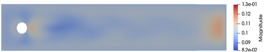
Fig. 11 Algorithm (3) solution when \epsilon = 0 for magnetic field at time T = 8.8 with \nu = 0.001 , \gamma = 0.1 and \Delta t = 0.001
