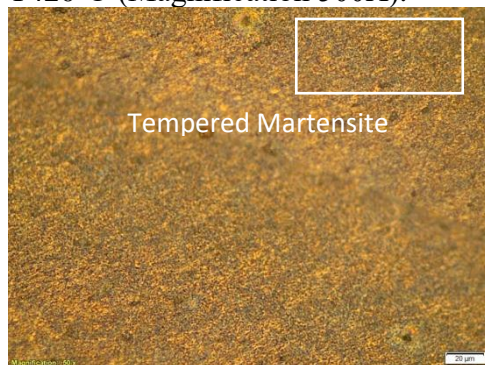
Figure 12. Microstructure of 855-T420-W (Magnification 500X).
