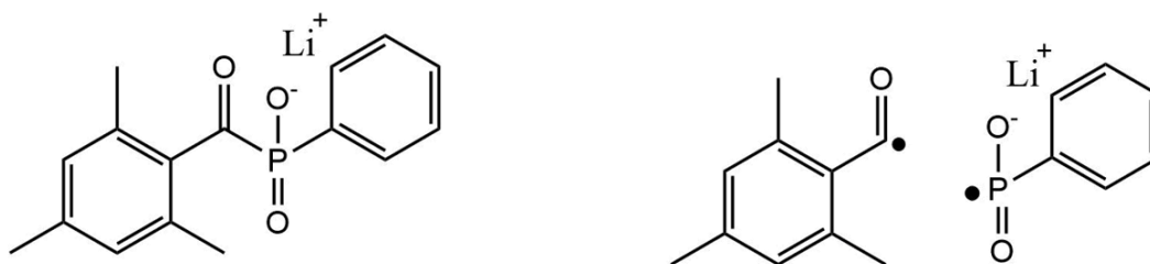
Figure 2.2: Radical generation upon light irradiation on LAP photo-initiator.
