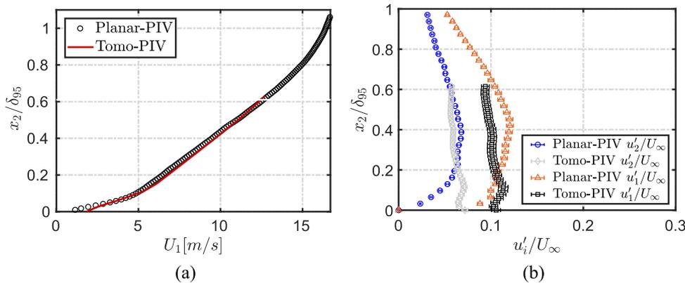
FIG. 6. Comparison of velocity profiles between the two different PIV experiments at RMP 26: (a) mean wall-tangential velocity  $U_1$  and (b) rms velocity components  $u_i'$  normalized by the inlet velocity  $U_\infty$ .
