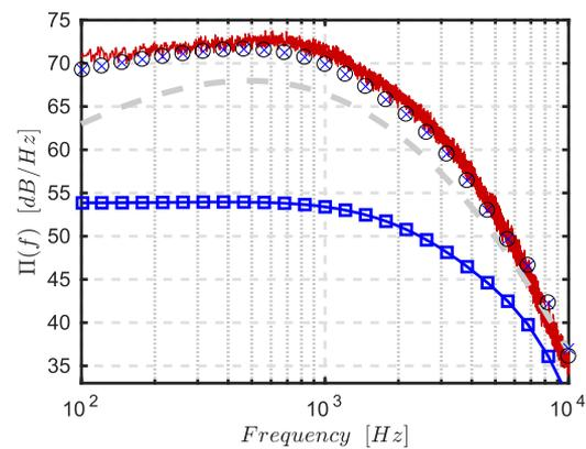
**FIG. 24.** Comparison of wall-pressure spectra models against experimental measurements at RMP 26. Legends: red solid curve—probe RMP 26; gray dashed curve—Rozenberg’s model; black open circle—MS term quasi-random sampling; blue crosses—MS term importance sampling; and blue curve with open squares—TT<sub>22,22</sub> quasi-random sampling.
