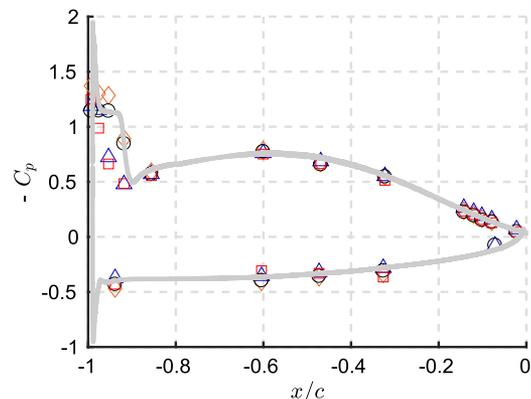
FIG. 4. Mean pressure coefficient  $C_p$  for the CD airfoil in different wind tunnel facilities. Legends: orange diamonds—V-Tunnel at TU Delft, black circles—anechoic wind tunnel facility at UdeS, blue triangles—anechoic wind tunnel facility at ECL [see Moreau and Roger (2005), for instance], red squares—wind tunnel facility at MSU [see Neal (2010), for instance], and gray curve—LBM DNS [see Sanjosé et al. (2011), for instance].
