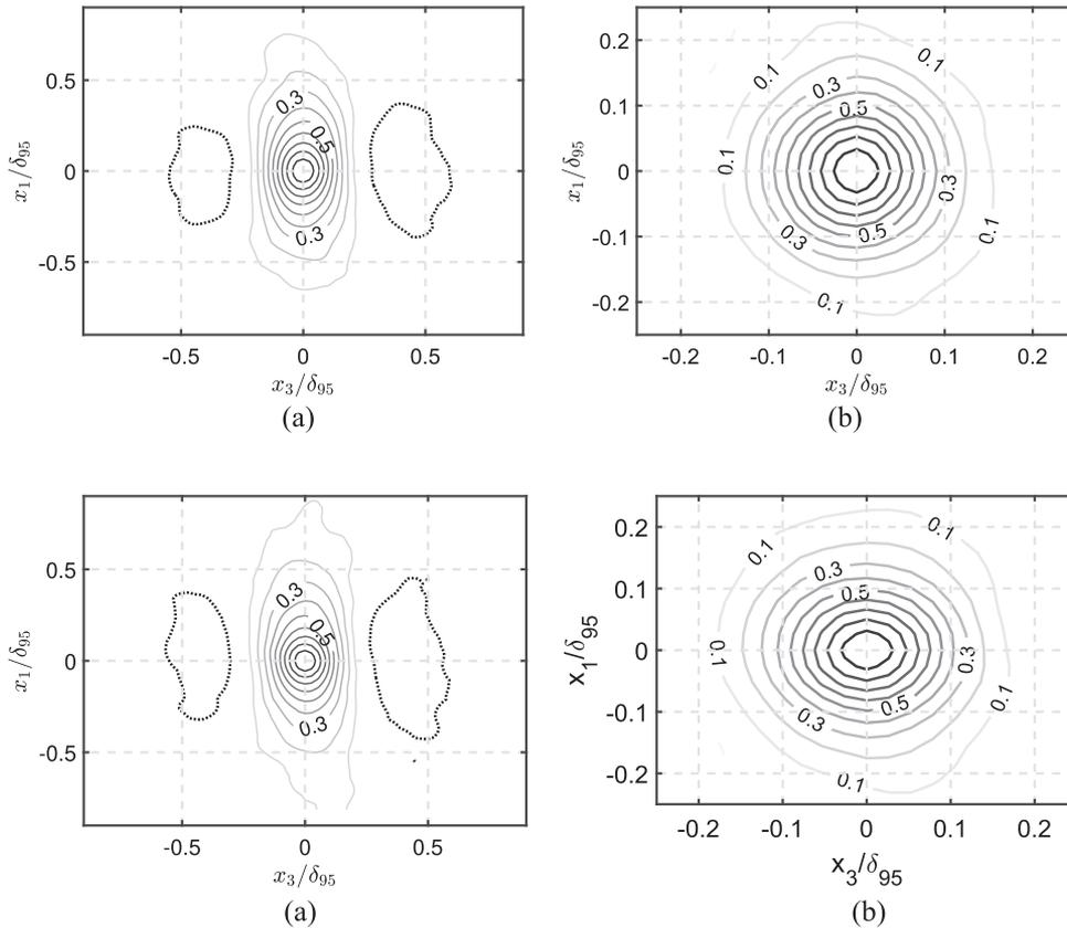
**FIG. 7.** Tomo-PIV second-order two-point zero time-delay correlation  $R_{ij}(x_1, x_1', 0.45 \times \delta_{95}, 0.45 \times \delta_{95}, x_3, x_3')$  in a plane parallel to the wall (iso  $x_2$ -cut) at RMP 26 ( $x_1/C = 0.98$ ): (a)  $R_{11}$  and (b)  $R_{22}$ . Color transition from the black curve to gray curve indicates decreasing values of correlation, and dotted curves indicate negative values.
