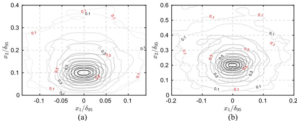
FIG. 19. Two-point correlation  $R_{22}$  from the PIV data (black solid curves) and anisotropy tuned model (black dashed curves) (a) at fixed point  $0.1 \times y/\delta_{95}$  and (b) at fixed point  $0.2 \times y/\delta_{95}$ . The color transition from the black curve to light gray curve represents decreasing correlation.
