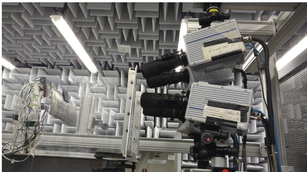
FIG. 3. Tomo-TR PIV setup.
