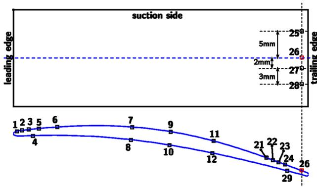
**FIG. 1.** Location of pinholes on the CD airfoil.
