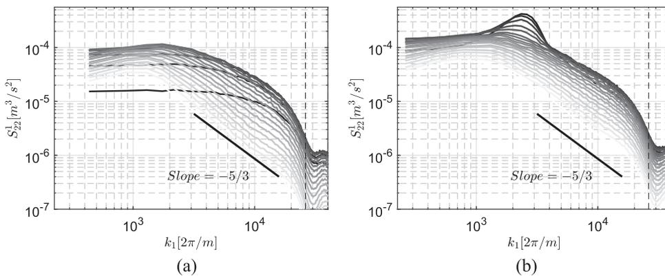
**FIG. 17.**  $S_{22}^1$  wavenumber energy spectra. (a) Measurement domain without the wake. (b) Entire measurement domain. Legends: The color transition from the black curve to light gray curve indicates fixed probe location close ( $x_2 = 0.037 \times \delta_{95}$ ) to the wall and away ( $x_2 = \delta_{95}$ ) from the wall, respectively. Black dashed curve—cutoff based on the interrogation window size.
