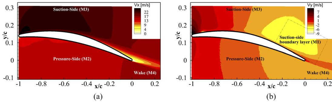
FIG. 5. Mean velocity contours around the airfoil in the laboratory reference frame: (a) streamwise velocity  $V_x$  and (b) transverse velocity  $V_y$ .
