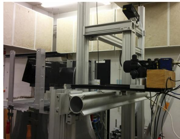
**FIG. 2.** Planar-PIV setup.
