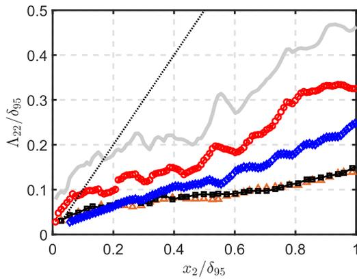
**FIG. 11.** Wall-normal velocity integral length scale  $\Lambda_{22}^{k\pm}$  at RMP 26. Legends: gray curve— $\Lambda_{ni22}^{2+}$ , red curve with circles— $\Lambda_{22}^{2+}$ , blue curve with diamonds— $\Lambda_{22}^{2-}$ , curve with orange triangles— $\Lambda_{22}^{1+}$ , and black curve with squares— $\Lambda_{22}^{1-}$ .
