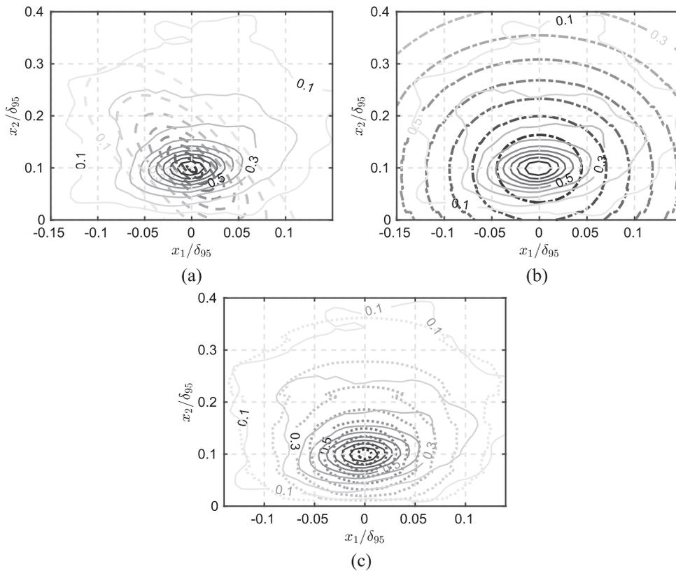
**FIG. 16.** Effect of wall-normal inhomogeneity on the wall-normal velocity correlation modeling. Black solid curves—PIV data. (a) Black dashed curves— $R_{22}$  model of Slama et al. (2018), (b) Black dashed-dotted curves— $R_{22}$  model of Grasso et al. (2019), (c) Black dotted curves—modified model of Panton and Linebarger (1974). The color transition from the black curve to light gray curve represents decreasing correlation.
