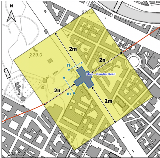
Figure 4. Extension of the area around the Mole-Giardini Reali station where the average parameters F , T , DF , I and GEO are evaluated.
