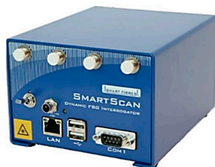
Figure 4. The Smart Scan interrogator used in the tests.
