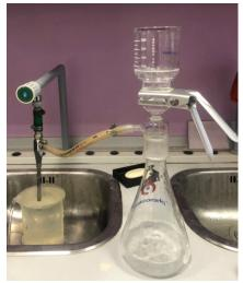
**2. Analysis of Microfibers:** After filtration and drying, each filter was weighed with a precision balance. An optical microscope was used to examine the GF filters. The microfibers were characterized using a Micro-FTIR at 700–4000 cm<sup>-1</sup>.
