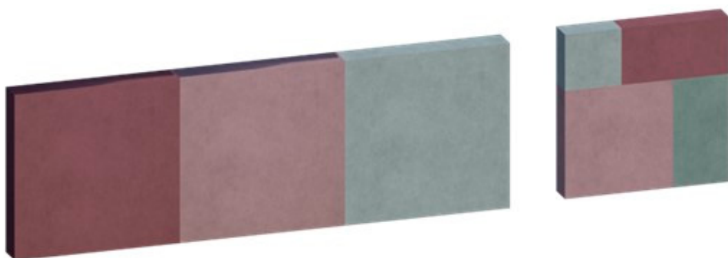
Figure 8. 3D modeling and rendering of the sound-absorbing panel ( O100l_{full} and Pattern-B) with pruning wood chips from olive trees used as the filling material and TNT as the containing membrane.
