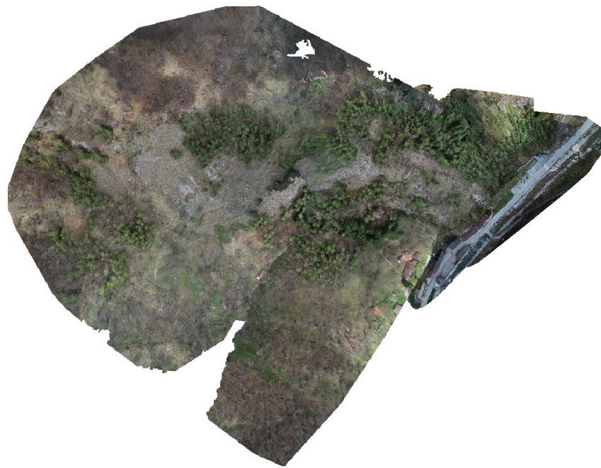
Figure 7. The final orthophoto, obtained merging all four image sets.
