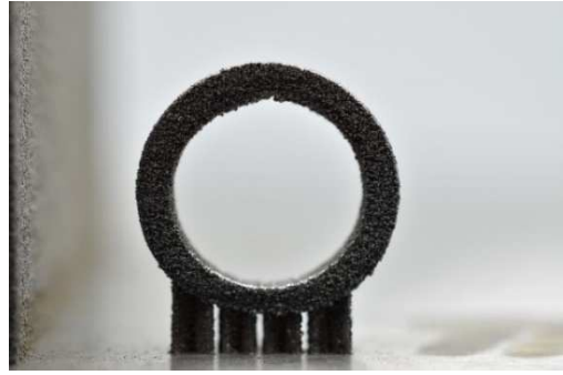
Fig. 3 - FeSi 2.9 Toroidal Sample: outer diameter 13.35 mm, inner diameter 9.58 mm and thickness 2.25 mm
