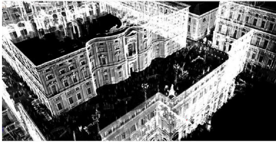
Figure 3: Point cloud views.
