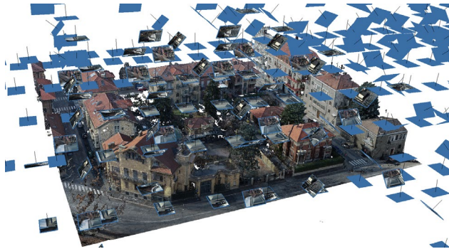
Figure 10. The photogrammetric flight plan on the urban square block, with the integration of nadir and oblique images.
